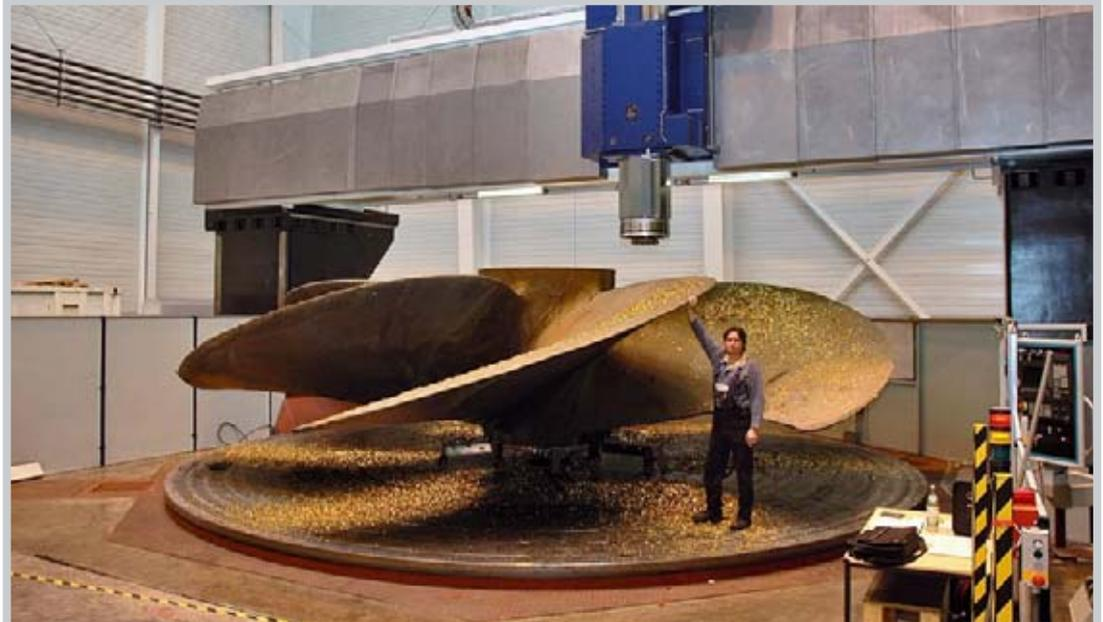
At MMG – the Waldrich Coburg portal milling machine 10500 FR-S2 allows the machining of propellers up to a diameter of 10500 mm.
